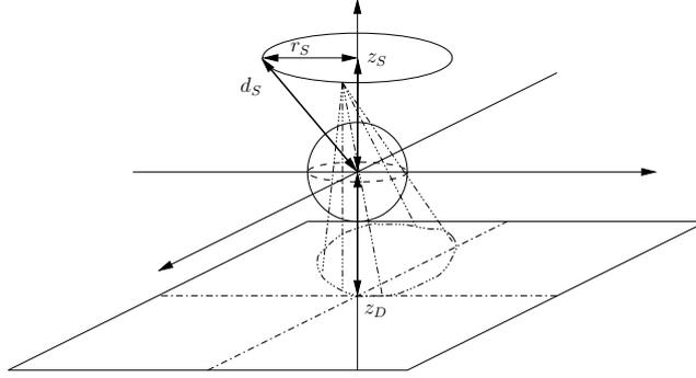
Figure 1: Circular tomography trajectory geometry.
